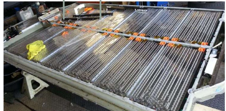
TESLA Model S 85 \text{ kWh: } 96 \times 4.19 \text{ V} = 402 \text{ V} 60 \text{ kWh: } 84 \times 4.19 \text{ V} = 352 \text{ V}
